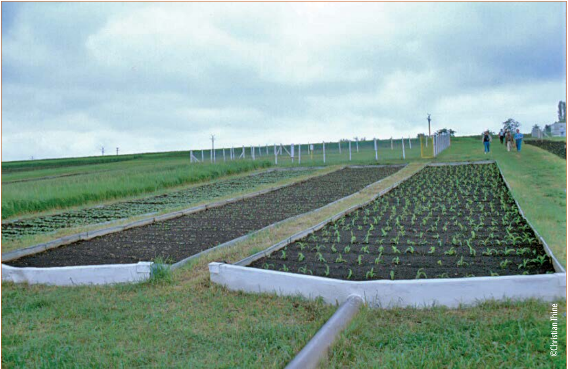
Figure 25: Standard erosion-runoff plots used to generate data for the Universal Soil Loss equation. Eastern Romania.
